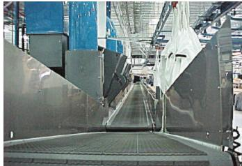
After a washer or a dryer has completed its cycle, the machine will look to see if there is a means to unload. The machine will send an invitation to be unloaded. If the conveyors "Belt Empty" input is on, the conveyor will send an invitation to be loaded. This will start the unload sequence.
